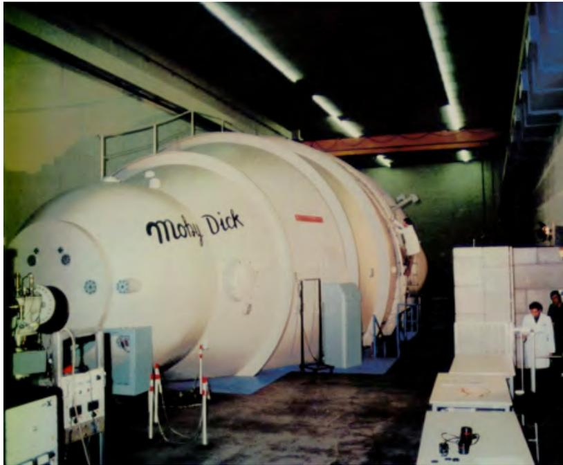
Figure 2: *The Tandem in the INFN National Laboratory of Legnaro (LNL), Italy, rated for more than 15 MV.*
